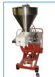
Optional electric scissor cart allows the operator to lower the machine to manually reload the hopper with product
