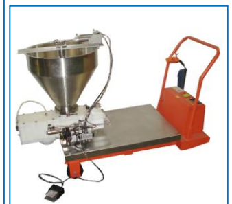
Optional electric scissor cart allows the operator to lower the machine to manually reload the hopper with product
