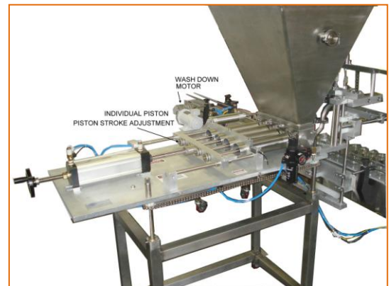
Rear view showing cylinders & pistons
