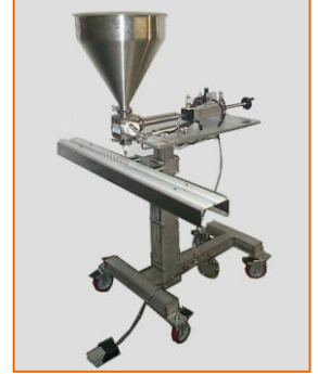
4 ft. s.s. container track
