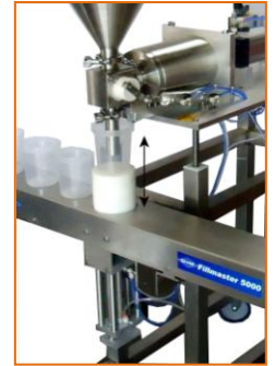
Container lift mechanism
