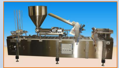
Cup filling and sealing machine
