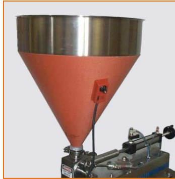
Silicone heater for hopper
