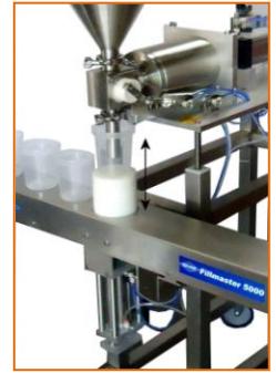
Container lift mechanism
