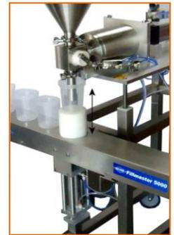
Container lift mechanism
