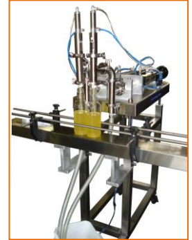
s.s. container track
